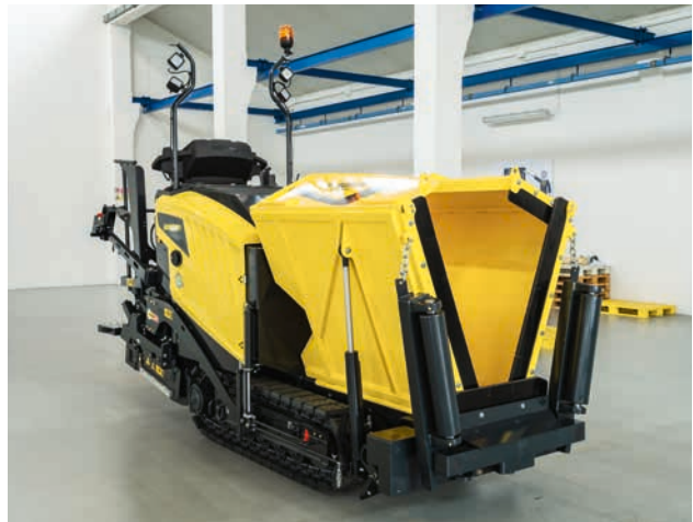
Long crawler tracks ensure dead straight paving.
