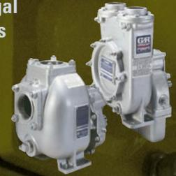
Power Take-Off pumps are designed for single saddle mounting with offset drive shafts that may be mounted in one of four positions to assist in alignment. These models are supplied with helical quiet-running gears, built for long life and available in right- or left-hand rotation.
