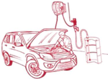
It is an automated system of interconnected devices that, as a whole, manage the fluid economy in a comprehensive manner. The terminal prevents unauthorized users and vehicles from taking fluids. It saves all information about a given fluid intake (employee, vehicle, date, quantity of fluid, etc.) and automatically sends data to the reporting software. The employee's role in such a system comes down to daily control of the system in the software and possible orders for ending fluids.
