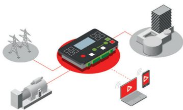
IT Controllo remoto via ethernet, rete 2G-4G e controllo posizione GPS EN Remote control via ethernet, 2G-4G network and GPS position control FR Commande à distance via Ethernet, connexion 2G-4G, et contrôle de position GPS
