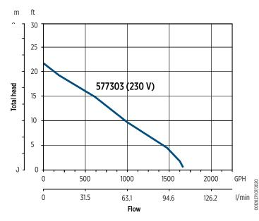
The hydraulic characteristics are guaranteed, according to ISO standard 9906, grade 3B
